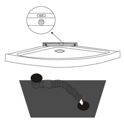
Connect the waste pipe of shower tray to the waste pipe in the floor.
